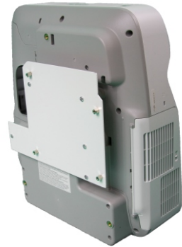
That's how should you place projector to screw it to fixing arm
