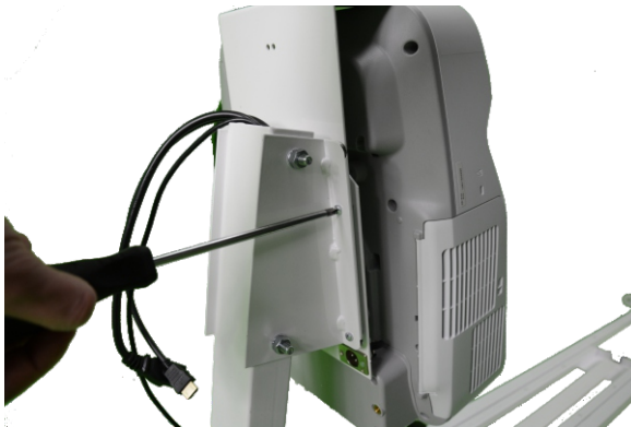
Montage of Epson projector with four M4x10 screws
